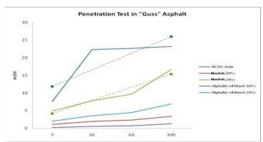
The most feasible resins were tested in an asphalt mix to see if the behavior was detectable in an asphalt mix. For this experiment a "Guss Asphalt" was used because this high binder containing asphalt gives a good indication of the bitumen properties.
